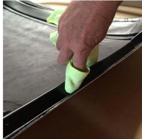
2. Remove the red backing from the window seals, and carefully and slowly press the seal onto the hard top surface you just prepped. Note: You will see some slight kinking around the corners, but this is normal and will not affect the quality of the seal (Photos below.) Full bond takes 72 hours.
