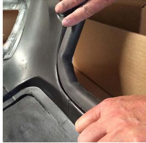
3. To seal the rear window, remove the window, then repeat step 1, prepping the area on the hard top around the window with tape primer. Allow it to dry.
